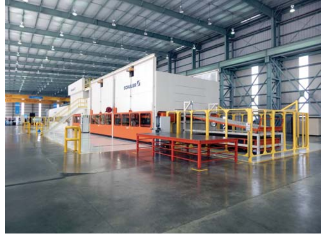
Schuler's new Tri-axis Transfer takes the parts from one die to the other, the interim storage becomes obsolete.
